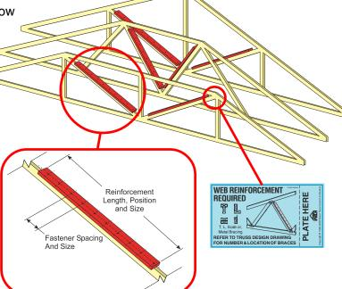
Refer to the Truss Design Drawing to get specific installation information on the web reinforcement. For future reference, you can request over-designed web material to reduce the number of web braces or web reinforcements required. The savings in labor and materials on the job site may offset the possible cost increase for the over-designed webs.
