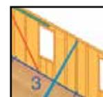
Stake each brace in ground, or attach securely to the floor deck.
