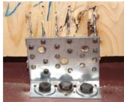
Figure 7: CLT shear wall bracket (Schneider, 2009)
