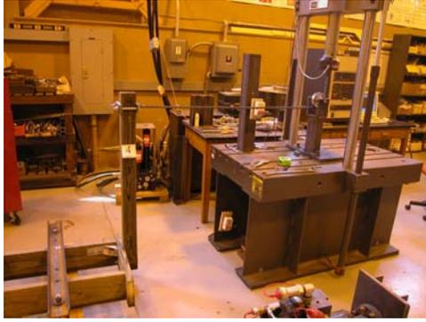
*Figure 2 Test set-up for rail posts showing roller chain and pulley to redirect force from test machine to top of post*
