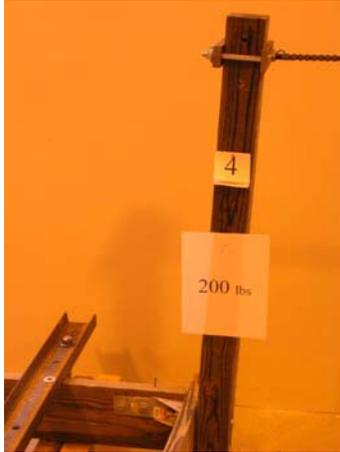
*Figure 11 The post loaded with the design load of 0.889 kN*
