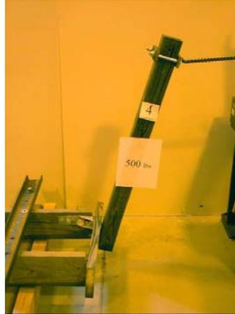
*Figure 12 The post loaded with 2.5 safety factor of 2.22 kN*
