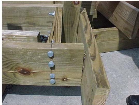
*Figure 7 Splitting perpendicular to the grain in the wood cleats*
