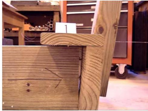
*Figure 5 Failure of screws in withdrawal from joists*
