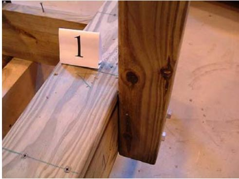
*Figure 4 Specimen with deck board and post*
