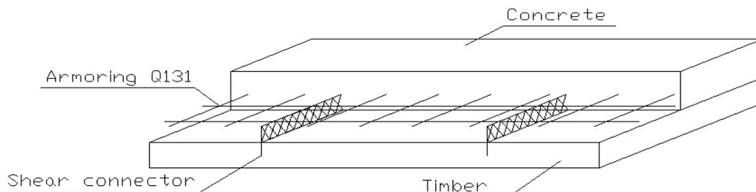
**Fig. 1** Structural elements of the wood-concrete composite system.
