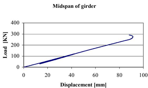
**Fig 8** Load vs mid-span displacement
