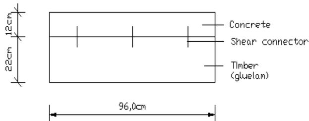
**Fig 6** Bending test specimen cross section
