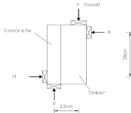
**Fig 4** Shear test set-up
