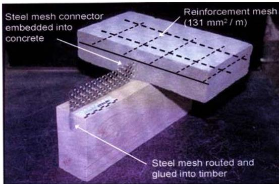
**Fig 3** Shear test specimen
