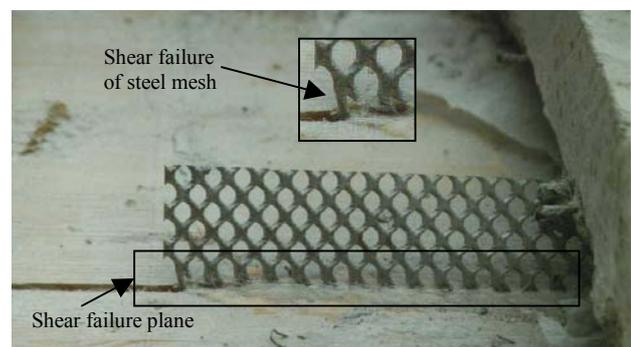
**Fig 9** Steel failure of beam specimen
