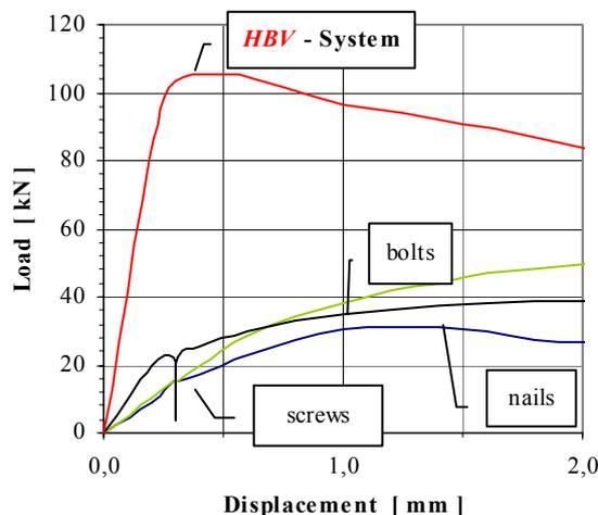
**Fig 2** Comparison of load-displacement curves
