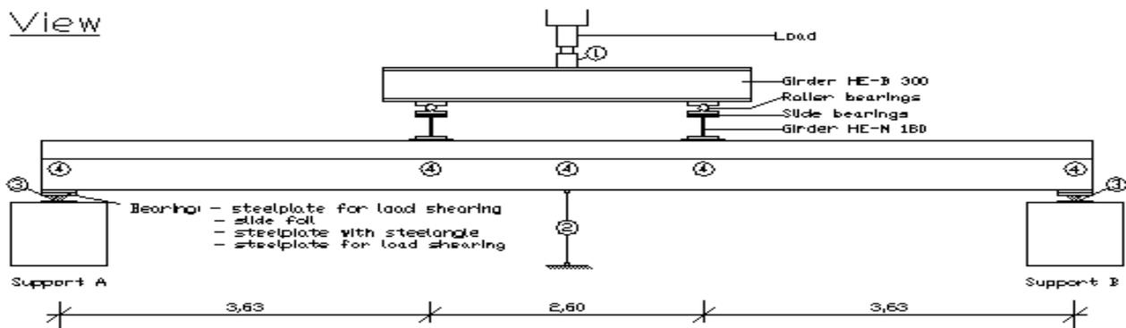
**Fig 7** Beam specimen test setup
