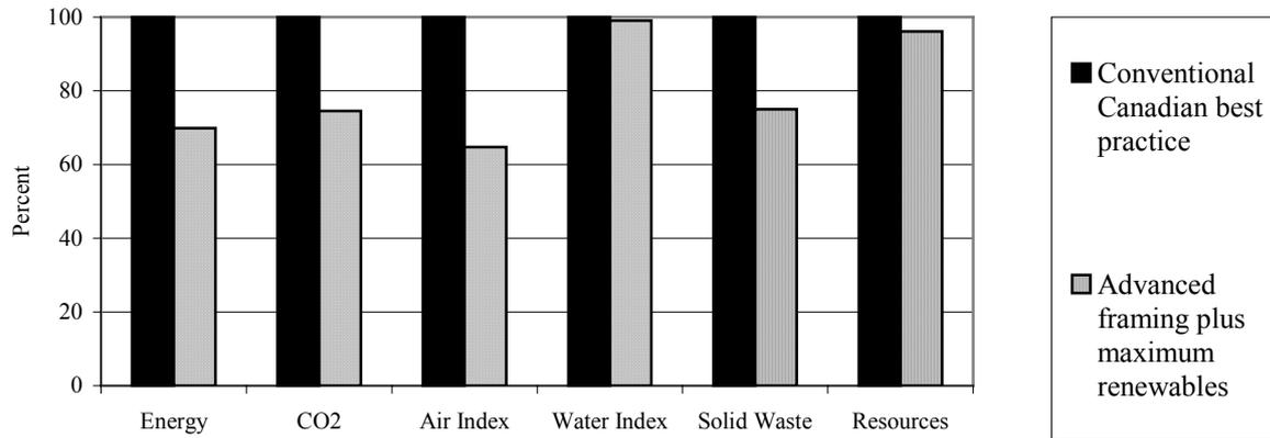
Figure 1: Comparative embodied LCA results for advanced framing with renewable siding and insulation versus a conventional house (the baseline).
